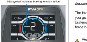
The FW7<sup>S</sup> EBS has the added advantage of an Electronic Braking System (EBS) for hill descent control.
