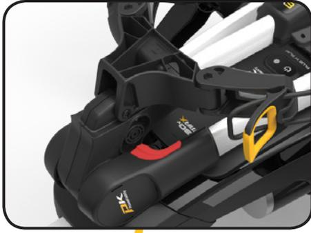
To open the frame, press the grey main lock button (highlighted in red) and lift the handle until the rear and upper joints click into place. Rotate To fold the trolley, reverse the process to fold so that the handle hook locks into the rear joint.
